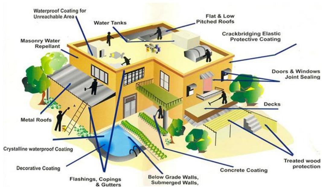
Figure 3. Complete waterproofing solution for a building
