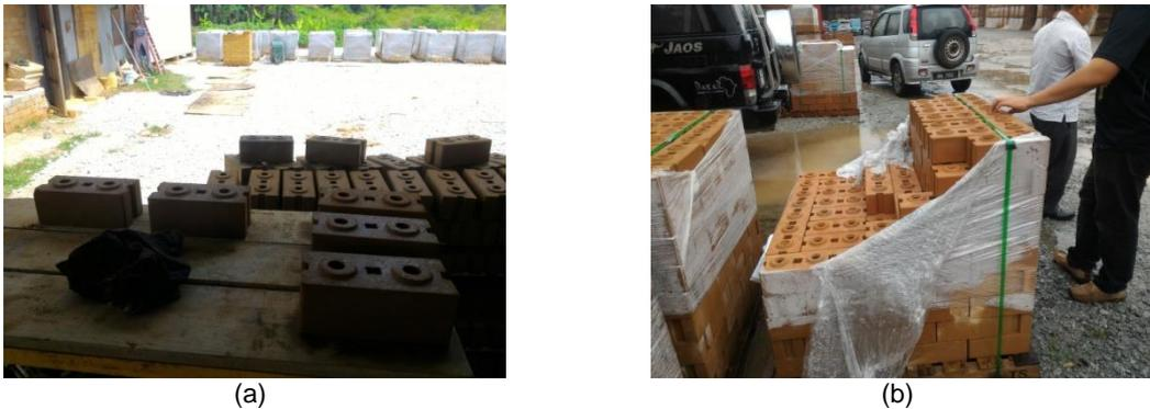
**Figure 1.** Physical form of Interlocking Soil Block manufacture by; (a) Company A, (b) Company B
