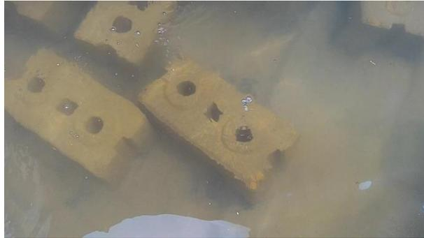
**Figure 8.** Density test of the blocks that have been performed by Company A
