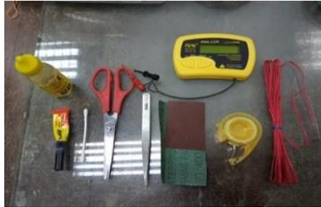
**Figure 4.** Strain Gage Attachment Equipment and Tools
