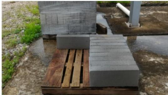
**Figure 2.** Physical form of Lightweight Block manufactured by Company C
