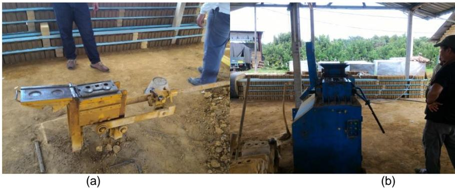
**Figure 3.** Type of machine that are used in Company A; (a) manual machine, (b) semi-auto machine
