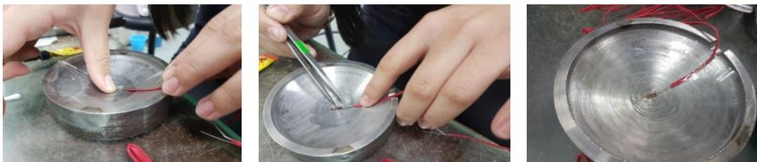
**Figure 6.** Attachment of Strain Gage to Metal Block
